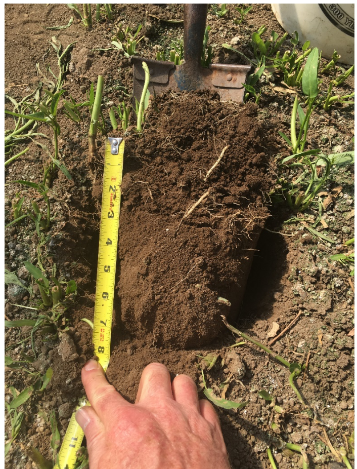
Figure 3. A V-shaped hole around 8 inches deep, and a soil slice section from one side of the hole. Photo by Drew Mather.
