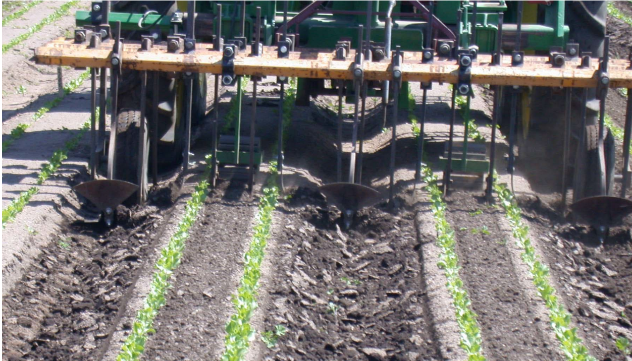
Figure 3. Row-crop cultivators may include combinations of bed knives, rolling baskets and duckfoot sweeps.
